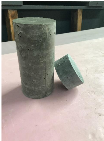
Figure 1. 4" x 8" Concrete Cylinders and 50mm Thick Concrete Sample
